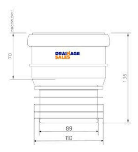
Technical Drawing of Specially designed SP140 connector for making connections of New PVC soil pipes with existing C.I. soil pipes.
