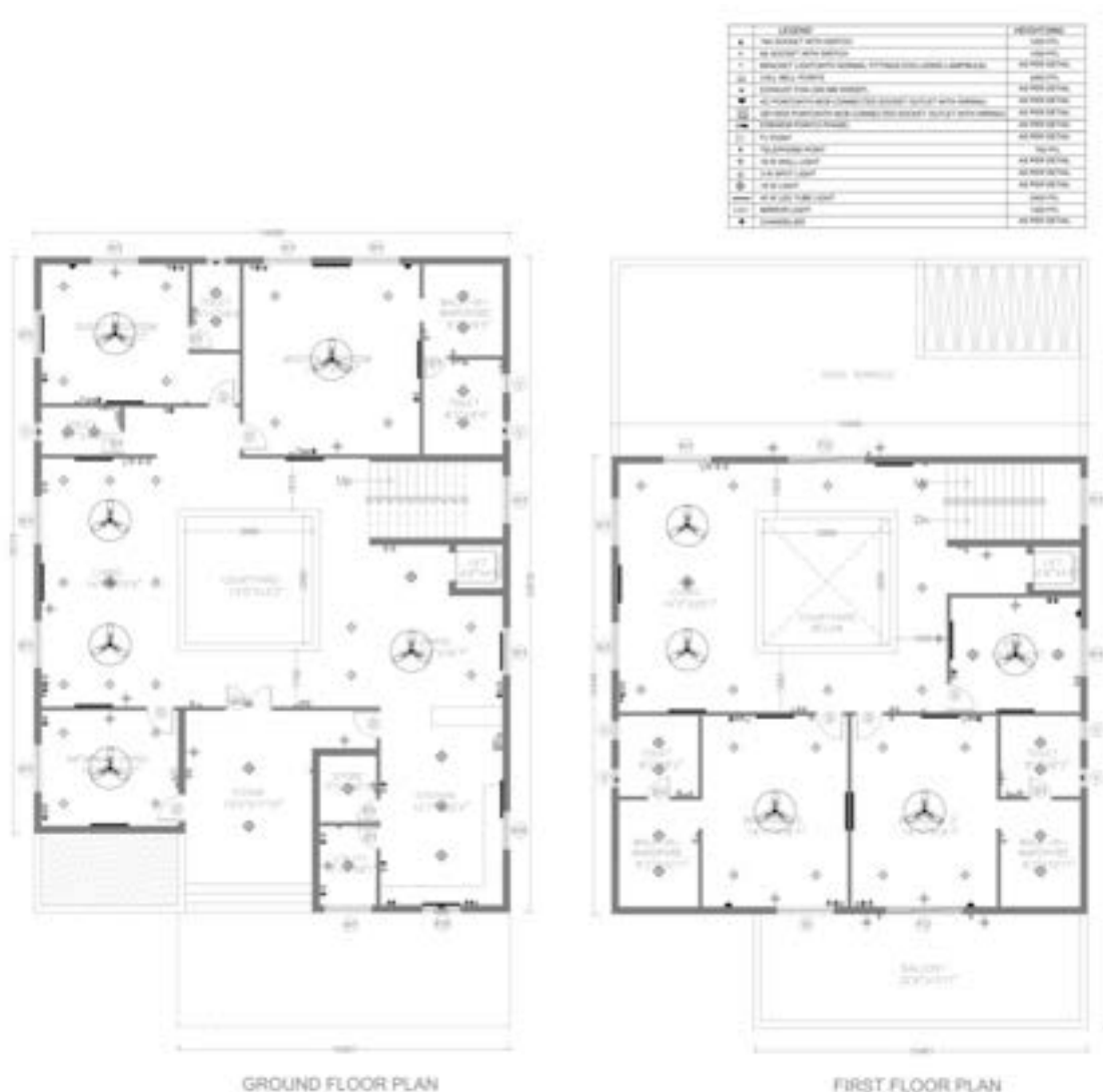
Figure 23 DMD Bungalow Floor plans with Electrical Installations
