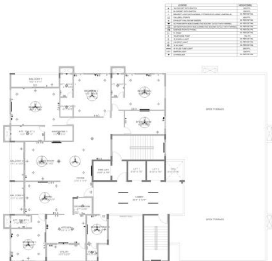
Figure 22 CGM Flats unit plan with Electrical Installations
