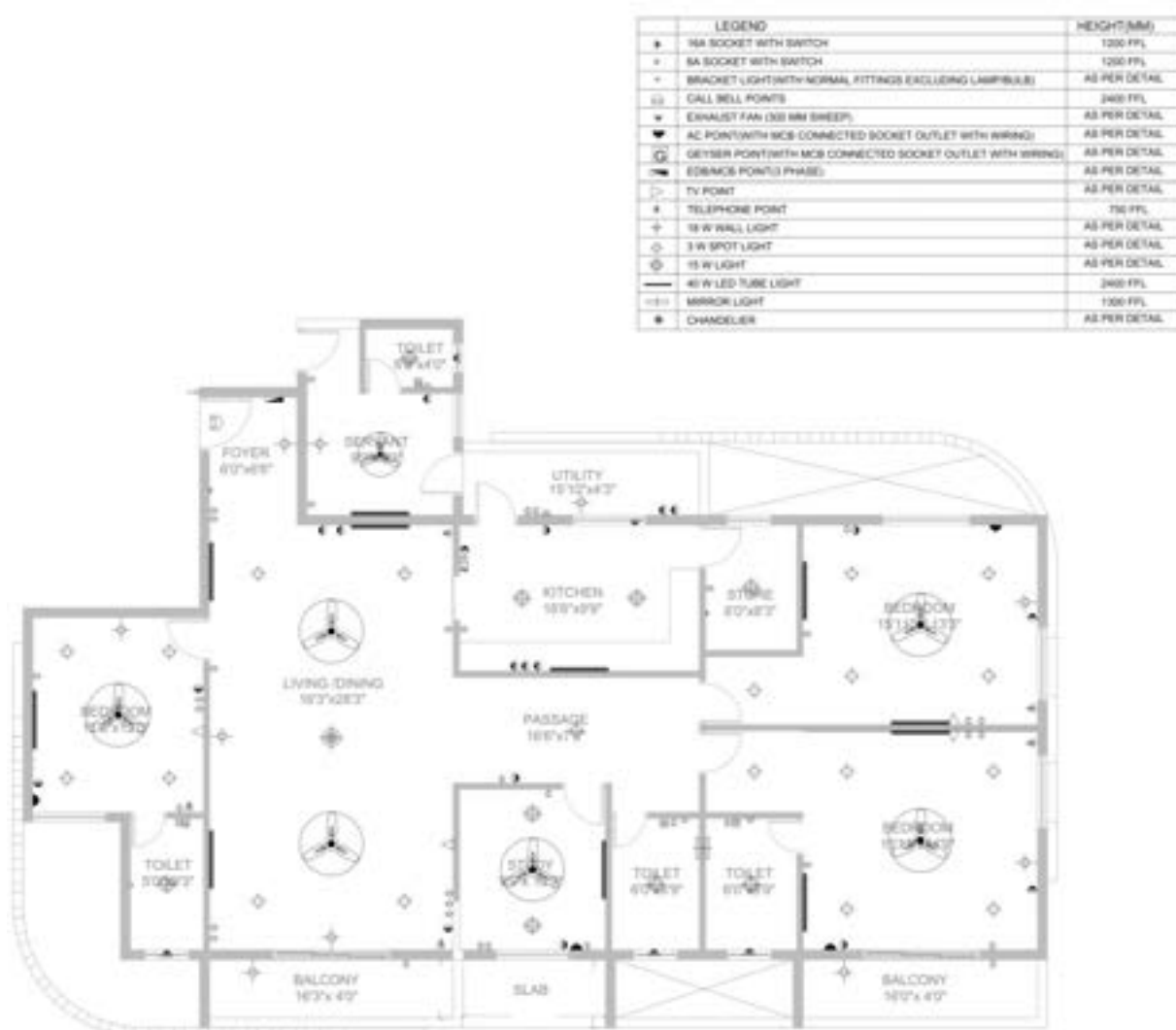
Figure 20 DGM Flats unit plan with Electrical installation
